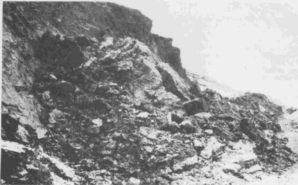
Close-up of black clay partly slickensided in shear, partly broken off in "granular chunks"
