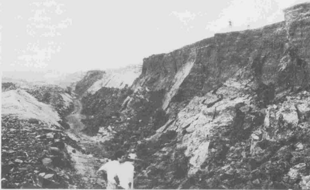
Views of slide scarp with stretches broken off in tension and areas slickensided in shear
